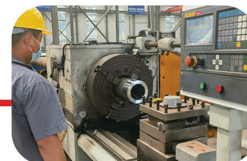
粗车 (加厚部位去除氧化脱碳层) Rough turning (Remove oxidation decarburization layer from thickened parts)
