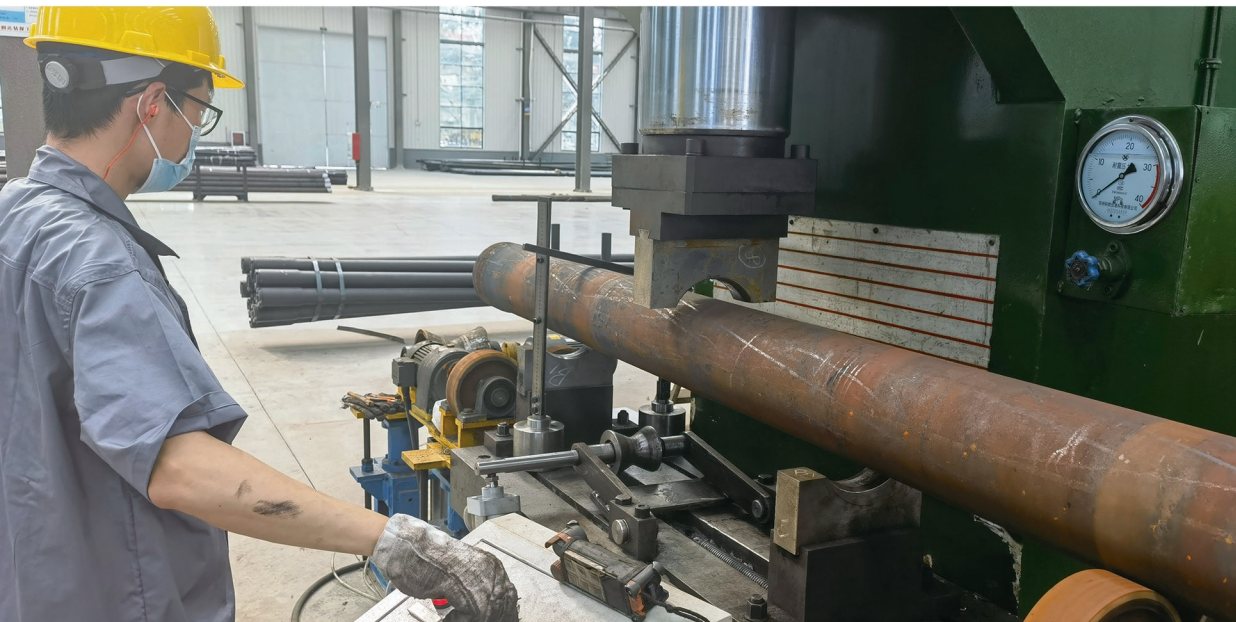
生产人员对每一根钻杆进行校直与检测 Production personnel straighten and inspect each drill pipe
