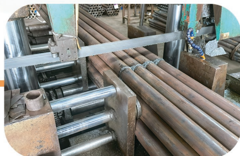
下料切割 (尺寸检测) Blanking and cutting (size inspection)
