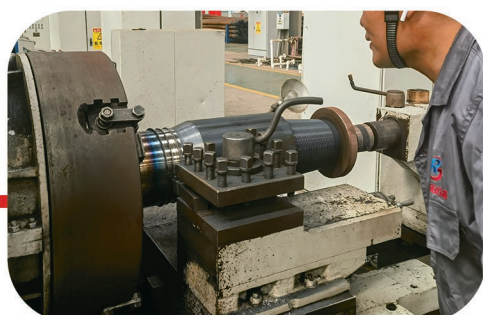
焊接处加工 (去除焊接挤压残骸) Welding processing (Remove welding extrusion debris)
