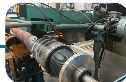
钻杆外修磨 (光洁度检测) Drill pipe outside polish (smoothness testing)
