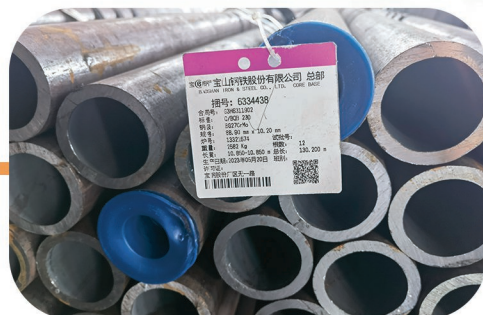
原材料 (钢管) (成分、规格尺寸检测) Raw material (steel tube) chemical composition analysis size inspection
