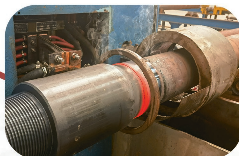
焊接处淬火 Welding quenching
