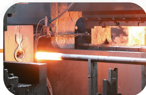
管端镦粗 (尺寸、成型检测) Pipe end thickening (size, shaping inspection)
