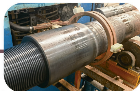
焊接处回火 (硬度检测、无损检测) Welding tempering (hardness test, non-destructive test)
