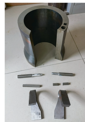
成品上取样，等待检测 Take samples from the finished product and wait for testing
