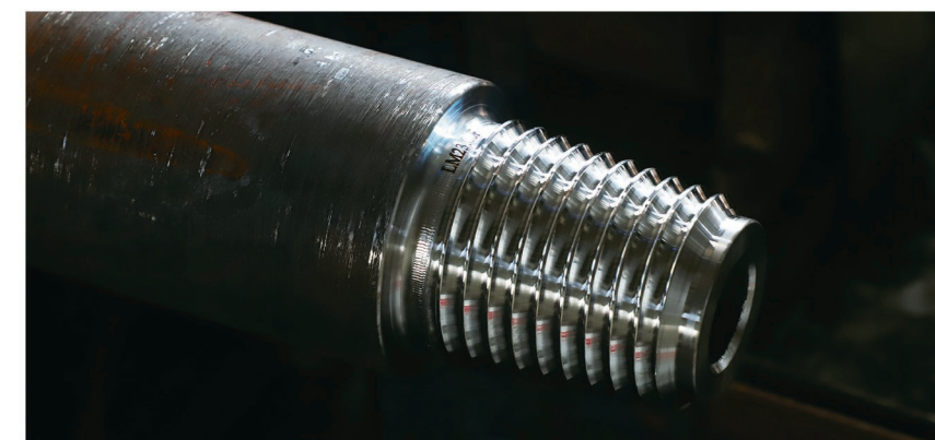
每一件合格的产品，都会通过激光刻字进行标识，确保了产品的可追溯性 Every qualified product is identified through laser engraving, ensuring product traceability
