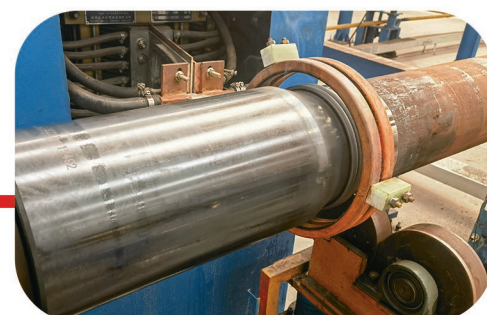
焊接处外圈回火 Welding outer ring tempering
