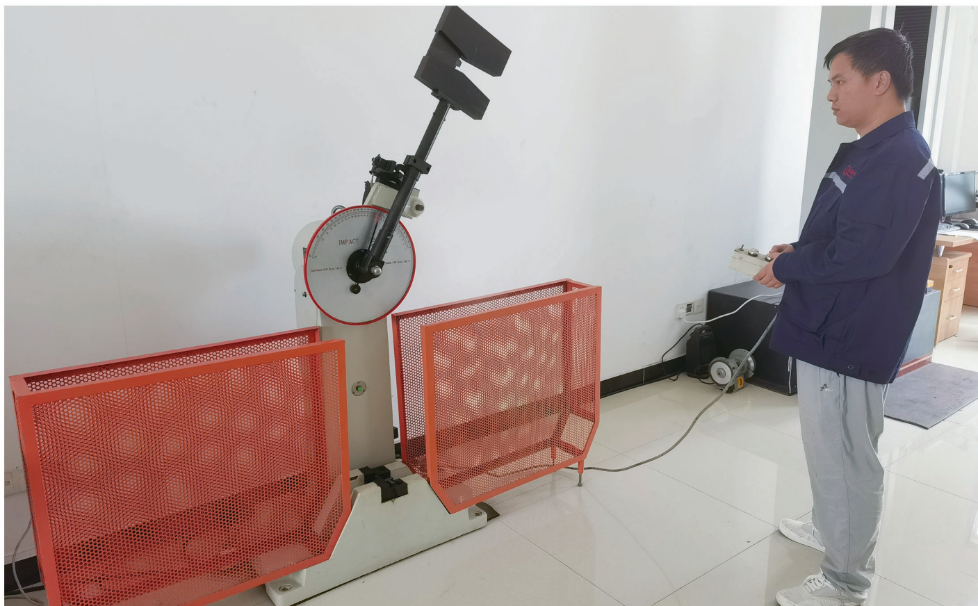
按照API标准进行冲击数据的收集 Collect impact data according to API standards
