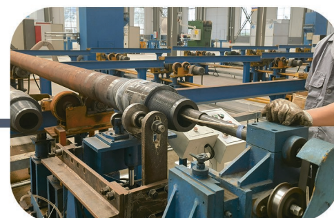
钻杆内修磨 Drill pipe inside polish
