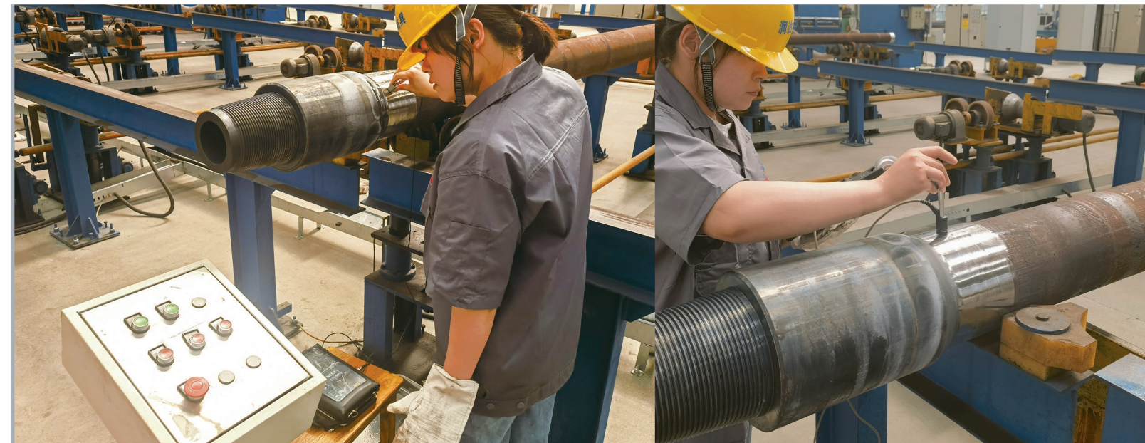
利用仪器进行无损检测 Using instruments for non-destructive testing
